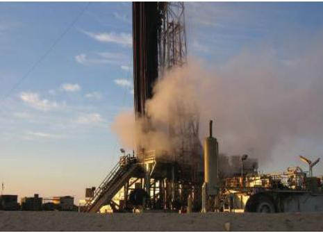
CWC was dispatched to a surface blowout that occurred while the rig was tripping out of the hole with a 3 1/2" tubing and a test packer. The well began to flow and the drilling crew made several attempts to install the kelly that were unsuccessful. The driller was unable to move the pipe in either direction as the packer had set prematurely at 2,400'. The flow became so strong after unloading the completion fluid that the rig crew was forced shut down the engines and abandoned the rig.
