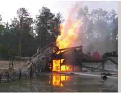
This well was drilling ahead at a depth of 4100' with 2000' of surface casing set. The rig hit a shallow gas zone and took a kick, resulting in a blowout and fire. The well was also producing a large volume of salt water. The drilling crew abandoned the rig and no injuries were sustained during the disaster. The rig and BOP stack were engulfed in flames.
